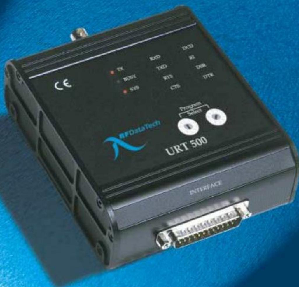
*The URT500 is an advanced, simplex/half-duplex, data radio designed to offer the UK utility market an easy upgrade path for systems using external modems, direct serial connections or a mixture of both. It has an audio interface for external modem connection and a serial port providing a true digital interface with speeds and data formats programmable to offer maximum compatibility with existing systems and other manufacturers products.*
